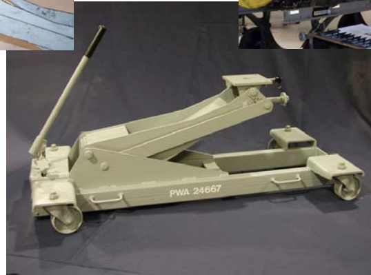
Model No. D-51403/PWA-24667 NSN 1730-00-005-5605 Use: Gear case handler
