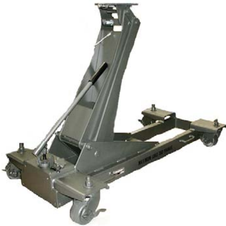
Model No. D-51403-2 NSN 1730-01-486-2539 Use: Ground support equipment for the F-22 Raptor
