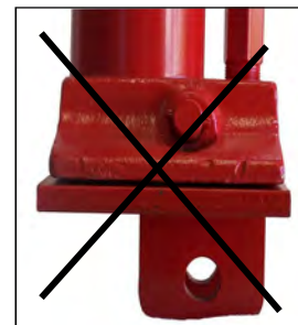
INCORRECT PLACEMENT OF BASE BRACKET
